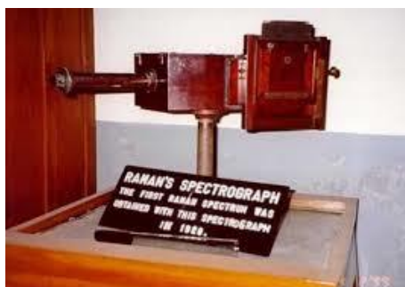
The first spectrograph used by Raman
