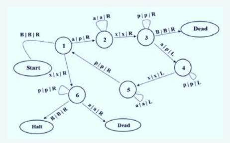
Figure 4: State Diagram of a Turing Machine which performs comparison of two strings.
