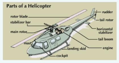
horizontal stabiliser and rudder can be there on the tail as shown in the figure. Horizontal stabiliser and the rudder are employed for stability. For safe landing of the fuselage, landing skids are attached to the lower side. Sometimes, the landing gear can have wheels for easy towing purpose .Of course, there are many more mechanical, electrical and electronic parts that are needed for its smooth operation and navigation.
