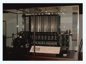
Figure 3(d) Babbage Difference Engine
